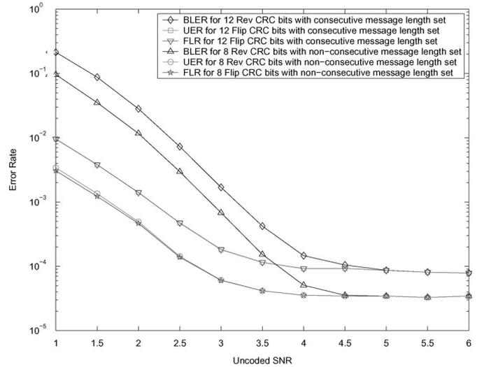
Fig. 9. Simulation results for the BLER, the UER, and the FLR with the same setting as in Fig. 5.
