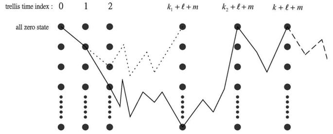
Fig. 2. Error-free path (solid line) of a convolutional codeword over its trellis diagram. Parameters  $k$ ,  $\ell$ , and  $m$  are the true message length, the number of CRC bits, and the memory order of the convolutional code, respectively.
