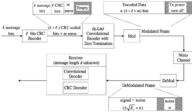
Fig. 1. Block diagram and frame structure of the *blind transport format detection using CRC* proposed in UMTS WCDMA standard. In the system, the receiver only knows the set  $\mathcal{K} \triangleq \{k_1, k_2, \dots, k_p\}$  of message lengths possibly used by the transmitter, but is not aware of the true message length  $k$ . The receiver, therefore, has to detect the true message length through the attached CRC bits with the help of convolutional decoder.
