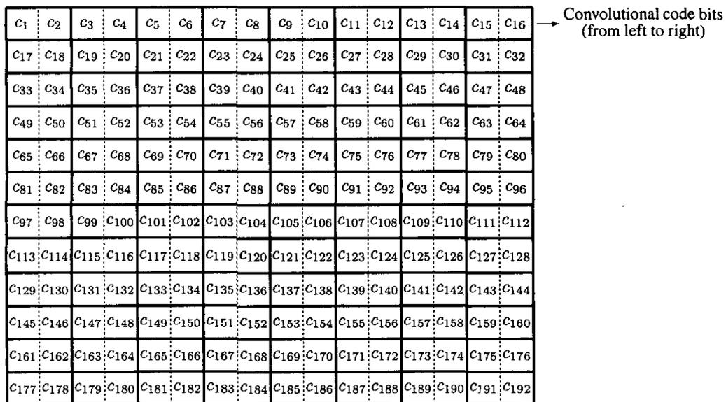
**Fig. 2.** (b) After de-interleaving, each 2-bit trellis branch for convolutional decoding is indicated by the flat rectangular in sequences from left to right.
