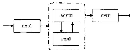
Fig. 1. A simplified block diagram of the Viterbi decoder
