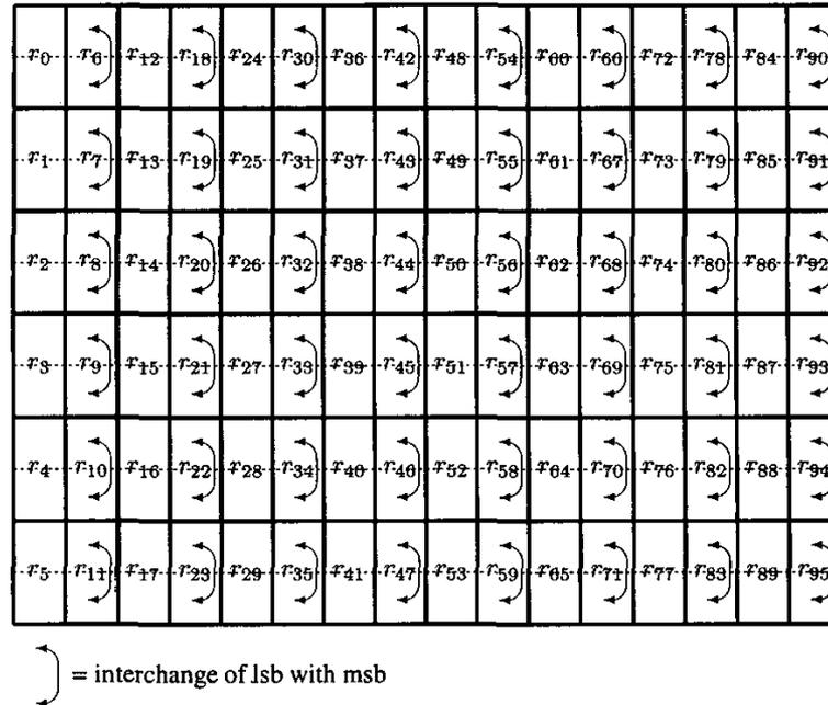
**Fig. 2.** (a) The received 16QAM quadrature components are indicated by a solid-lined upright rectangular; each column consists of 6 quadrature components. The de-interleaver should then exchange (the weights of) the least significant bit and the most significant bit of the quadrature components for those columns indicated.
