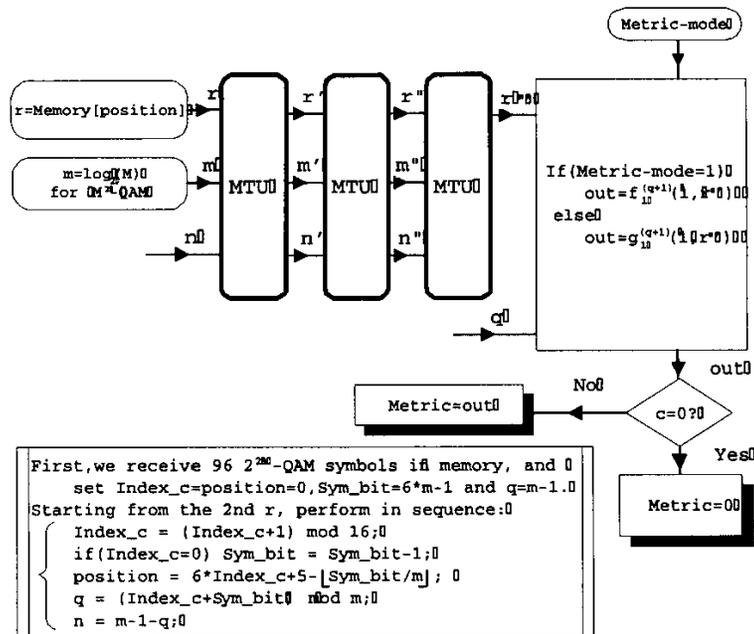
**Fig. 3.** A dual-mode BMU architecture with  $(m_{\max} - 2)$  MTU's can perform the bit metric evaluations for  $2^{2m}$ -QAM, where  $2 \leq m \leq m_{\max}$ . Here,  $m_{\max} = 5$ . All the constants in the formulas of Index\_c, Sym\_bit and position, such as 5 ( $= 6 - 1$ ), 6 and 16, are set because of the  $6 \times 16$  interleaver block used in IEEE 802.11a/g standard.
