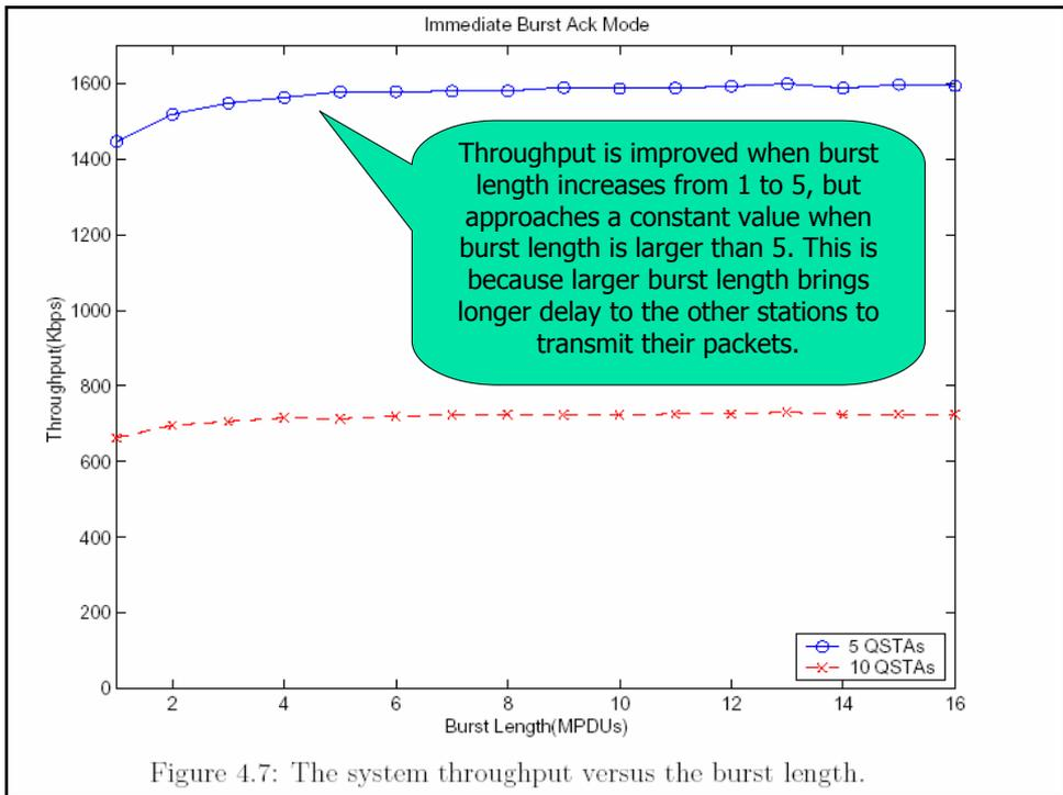
Figure 4.7: The system throughput versus the burst length.
