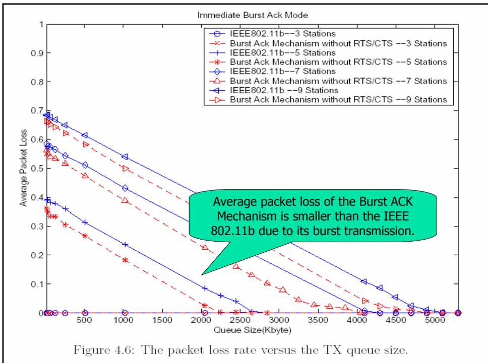
Figure 4.6: The packet loss rate versus the TX queue size.
