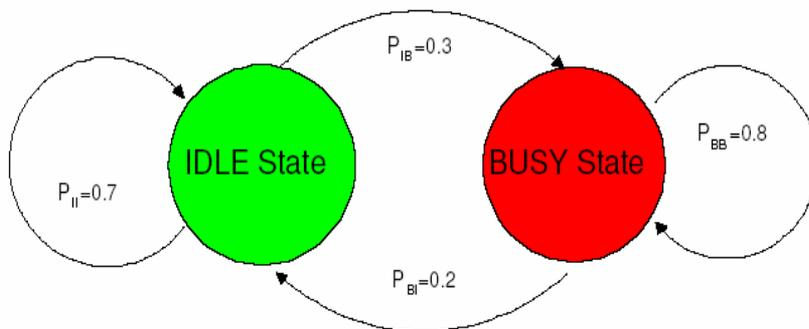
Figure 3.1: The Markov-Modulated Poisson Process.
