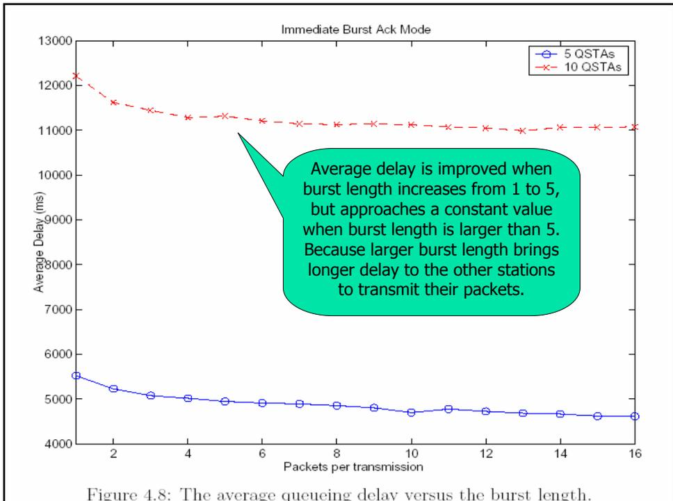
Figure 4.8: The average queuing delay versus the burst length.
