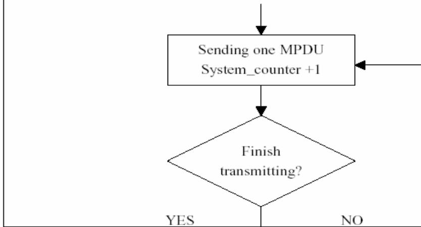
Figure 3.3: The Simulation Flow Chart of the EDCF.
