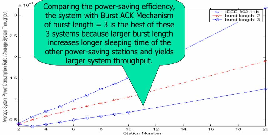
Figure 4.14: Average system power consumption ratio over average system throughput versus the number of QSTAs.
