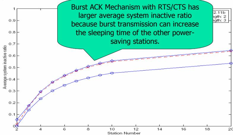
Figure 4.13: Average system inactive ratio versus the number of QSTAs.
