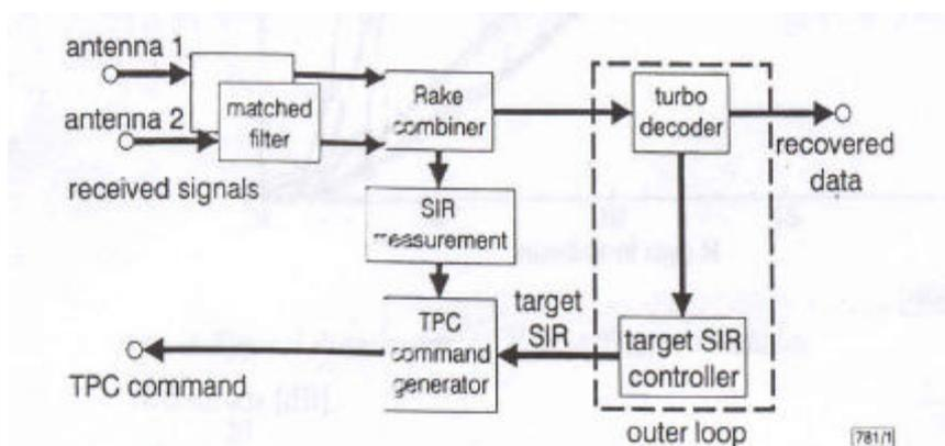
Fig. 1 Closed-loop fast TPC for turbo-coded W-CDMA receiver
