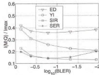
Figure 5. Mutual information between the BLER and the desired metrics vs. the averaged BLER. The mutual information is normalised to the amount of information in a binary symmetric channel (BSC).
